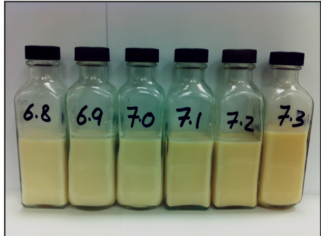
Fig 3. Heat stability of sterilised whole camel milk proteins containing sodium phosphate at a concentration of 1 mmol L -1 after adding NaOH to adjust the pH up to 7.3. No sedimentation and separation in proteins was noticed in camel milk directly after sterilisation process.
